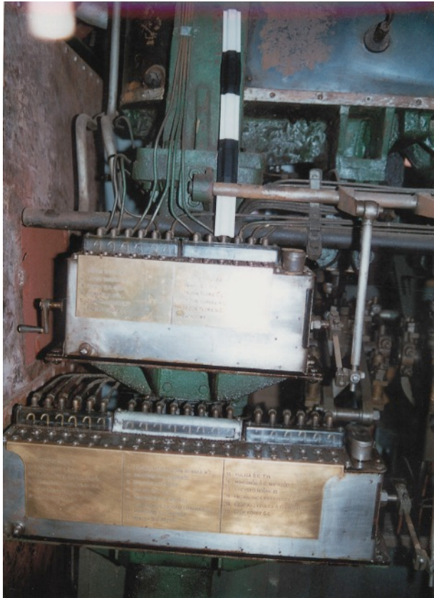
Above: The high and intermediate lubricators on the left and the low pressure on the right. Below: The high and intermediate cylinder reversing gear.
