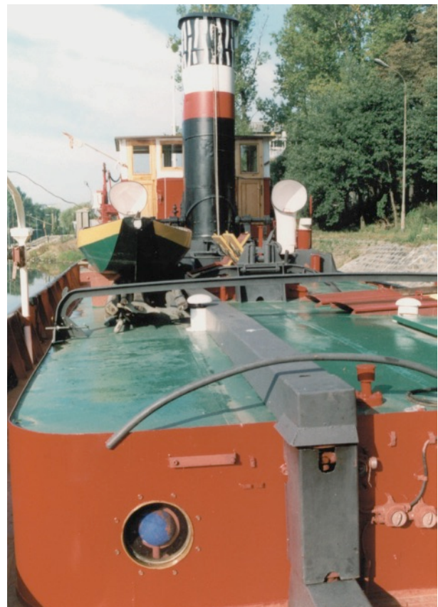
The steering drive which needs checking and cleaning so that the gears and shafts operate smoothly.
